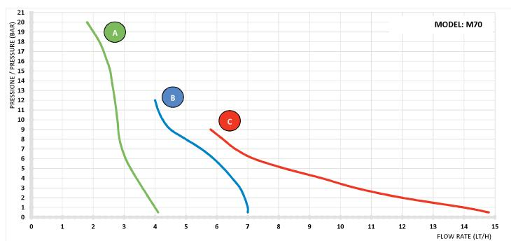
The above data are referring to tests made with water at room temperature. Values may vary by 10%.
