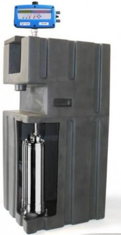
Hydrofix water pressure booster is an automatic solution for both domestic and commercial premises with low water pressure or flow. The self-contained system is compact, silent, easy to install and has a type AB air gap to comply with water authority regulations. Water from the mains or private water supply is stored in the tank which also houses a submersible pump. A built in flow sensor prevents the pump from running dry and automatically re-sets once the water level recovers.
