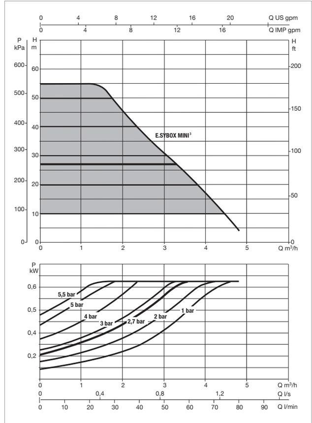
The performance curves are based on the kinematic viscosity values = 1 mm<sup>2</sup>/s and density equivalent to 1000 kg/m<sup>3</sup>. Curve tolerance according to ISO 9906.
