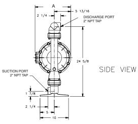
BOTH SUCTION AND DISCHARGE PORTS ARE AVAILABLE WITH 2" BSPT TAPERED THREADS
