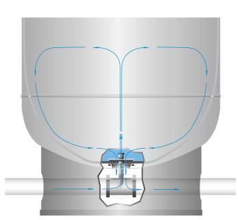
Flow-Thru<sup>™</sup> technology assures total recirculation of the tank's water content
