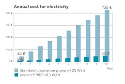
High efficiency circulator ecocirc® PRO saves energy, reduces environmental pollution resulting from CO<sub>2</sub> emissions and allows the customer to save money. The cost comparison of a standard circulator of 25 Watt and an high efficiency circulator ecocirc<sup>®</sup> PRO 15-1 of only 3 Watt power consumption clearly shows the difference.
