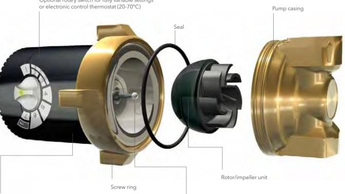
Stator/Pump motor with ECM technology The model with an electronic control thermostat (model number with "R") allows fully variable adjustment of the desired water temperature. At temperature the pump will switch off. This further reduces the energy consumption costs of the pump, the radiation losses in the circulation pipework and the energy requirements for the supply of warm water.
