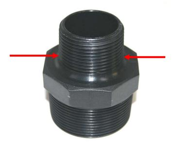
To accurately identify any BSPP or BSPT fitting, measure from one side of the thread to the other and refer to the chart above. EG: If the fitting measured 33.249mm across, it is a 1" BSP fitting and you would refer to it as a 1" BSP fitting. A 2" fitting would measure 59.614mm across the threads, it is still called a 2" BSP fitting.
