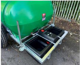
**CHASSIS** Constructed from 5mm pressed steel section fully welded with a 100 x 50 R.S.C 'A' frame drawbar and a front standplate.
